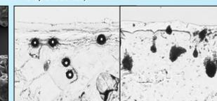
Pic.6: Comparison of particle penetration: a) 48µm polystyrene; b) SFD - Formulation 4
